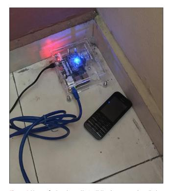
**Figure 2** Photo of a Raspberry Shake (RS) seismometer installed at a host located in Port-au-Prince. The RS is lying on the floor in a corner of their living room, behind a piece of furniture that hosts a TV and various electronics. The mobile phone gives the scale. The connection to the electricity (black cable) and the internet router (blue cable) can be seen.
