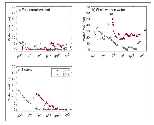
Figure 8 Example of summer relative water level position (cm) at (a) an ephemeral wetland using a groundwater well, (b) shallow open water wetland using a staff gauge, and (c) swamp using a groundwater well in 2017 and 2018.
