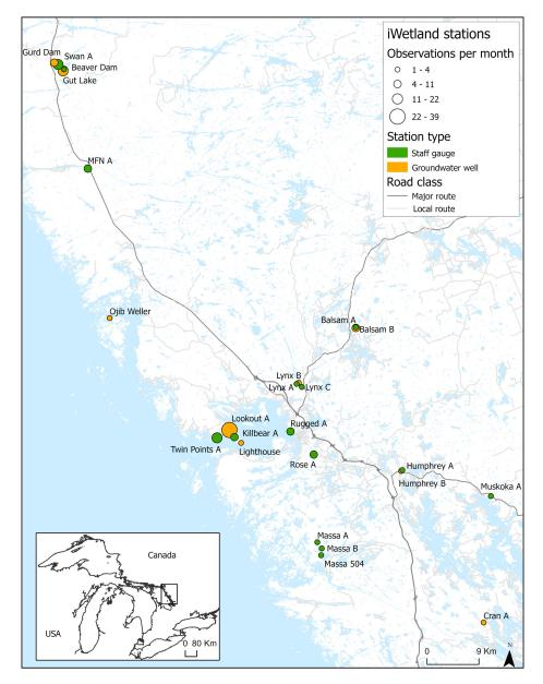
**Figure 3** The 24 iWetland stations span ~150 km along Georgian Bay in South-Central Ontario, Canada. The stations consist of 15 surface water monitoring sites (staff gauge) and 9 groundwater monitoring sites (groundwater well). iWetland stations were active for 1–4 years between 2016–2019 (See Supplementary File 5: Table S1). Waterbody and road shapefiles licensed under the Open Government Licence – Ontario.
