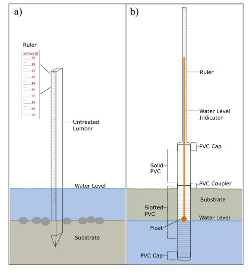
Figure 1 Diagram of (a) the staff gauge and (b) groundwater well iWetland stations.
