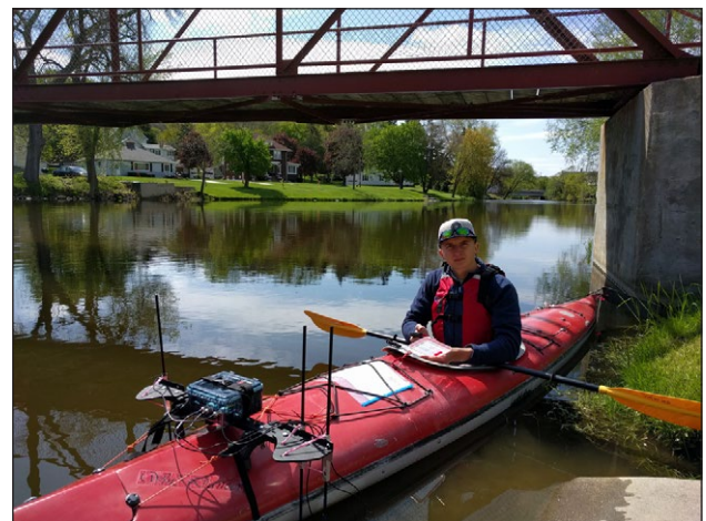
Figure 3: Prototype installed on the front of a kayak with flexible probe mounts. Photo by Eric Compas.
